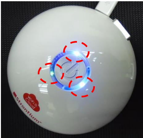
3 rd LED lighted - Charging
