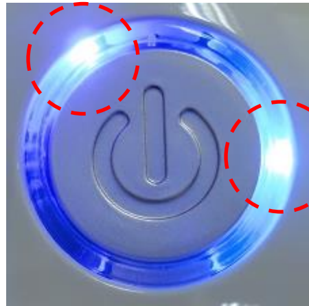
2 nd LED lighted and blinking - WiFi active
